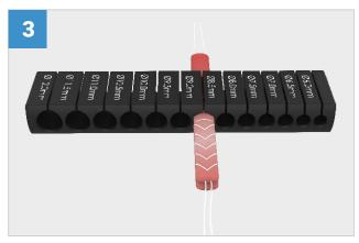
Fold up the graft and measure the diameter using the Graft sizer The graft should moderately pass through the hole, not too tightly not too loosely.
