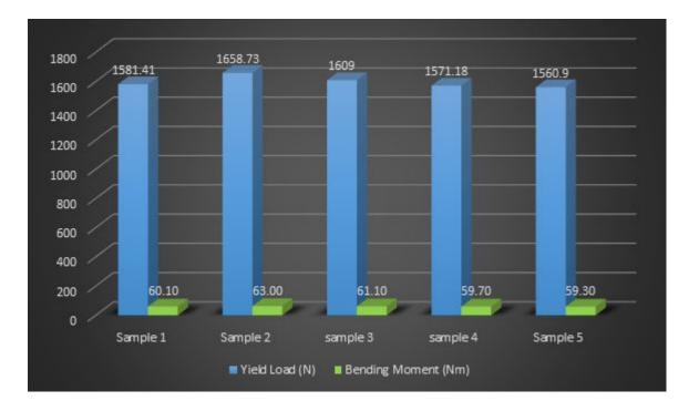
The Expert Tibia Nail Manufactured by M/S Auxein Medical Pvt. ltd. tested as per the test method described in ASTM F1264 for four point bend testing in order to determine the Yield load (N) as well as bending strength under the flexural loading.
