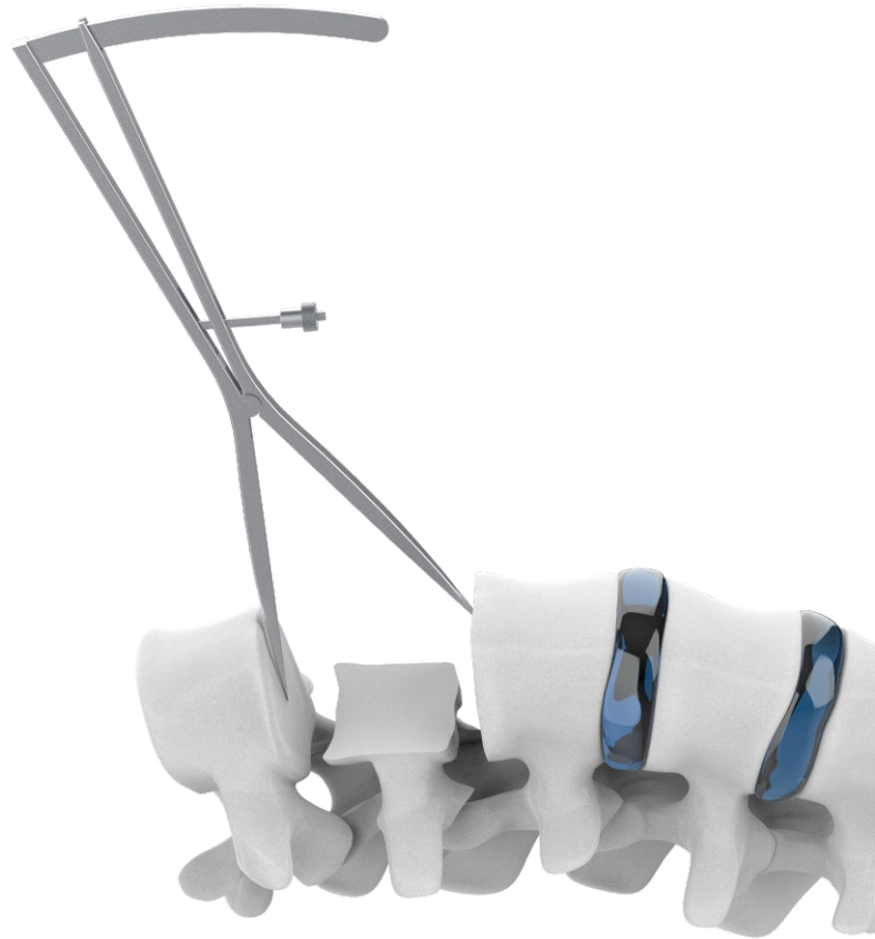
Confirm the height of the defect in situ by measuring from the posterior aspect of the motion segment(s).
