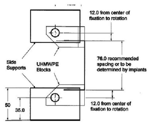
This test series was conducted to determine the torsional performance of Spinal System devices including hybrid construct of Auxein Medical as per ASTM F1717.
