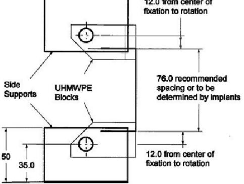
This test series was conducted to determine the torsional performance of Spinal System devices including hybrid construct of Auxein Medical as per ASTM F1717.
