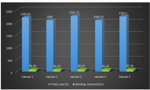
The Konzept Femur Nail Manufactured by M/S Auxein Medical Pvt. ltd. tested as per the test method described in ASTM F1264 for four point bend testing in order to determine the Yield load (N) as well as bending strength under the flexural loading.
