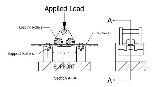
The Metallic Bone plates Manufactured by M/S Auxein Medical Pvt. ltd. tested as per the test method described in ASTM F1717.
