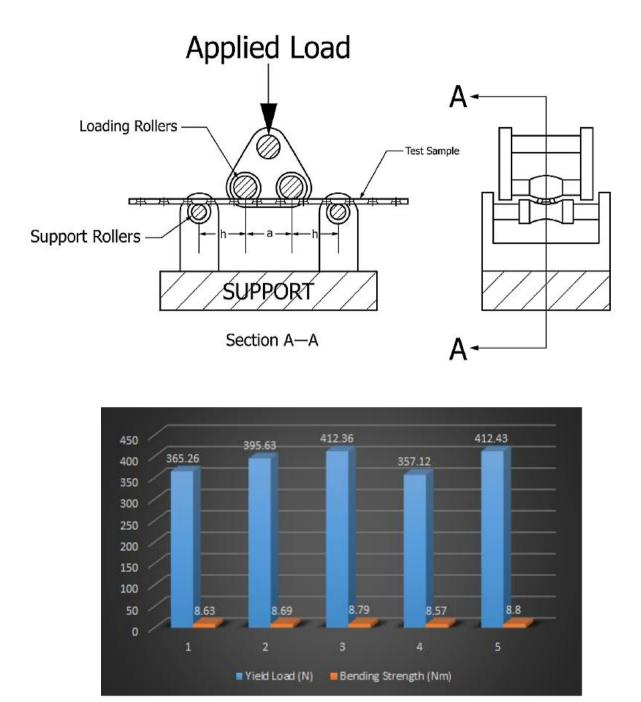
The Metallic Bone plates Manufactured by M/S Auxein Medical Pvt. ltd. tested as per the test method described in ASTM F382-17 for four point bend testing in order to determine the Yield load (N) as well as bending strength under the flexural loading.
