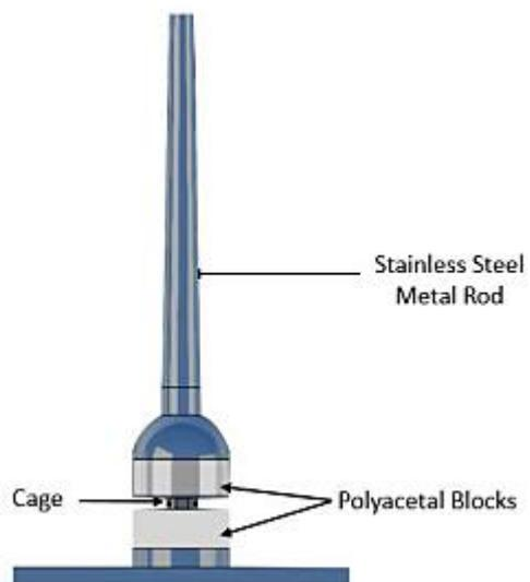
The spinal cages Manufactured by M/S Auxein Medical Pvt. ltd. tested as per the test method described in ASTM F2077.
