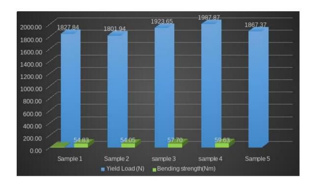
The JIN Type Tibia Nail Manufactured by M/S Auxein Medical Pvt. ltd. tested as per the test method described in ASTM F1264 for four point bend testing in order to determine the Yield load (N) as well as bending strength under the flexural loading.
