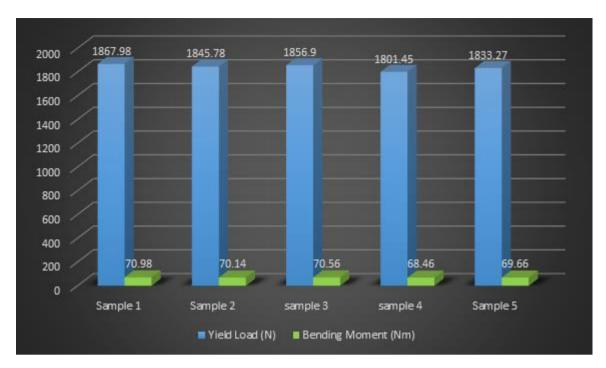
JIN Type Femur Nail Manufactured by M/S Auxein Medical Pvt. ltd. tested as per the test method described in ASTM F1264 for four point bend testing in order to determine the Yield load (N) as well as bending strength under the flexural loading.
