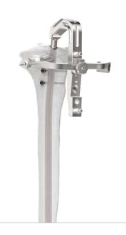
Insert the screw measuring gauge (520-041) through the protection sleeve and the required  $\emptyset$ 4.8mm Locking bolt length is measured from the marking on the measuring gauge.
