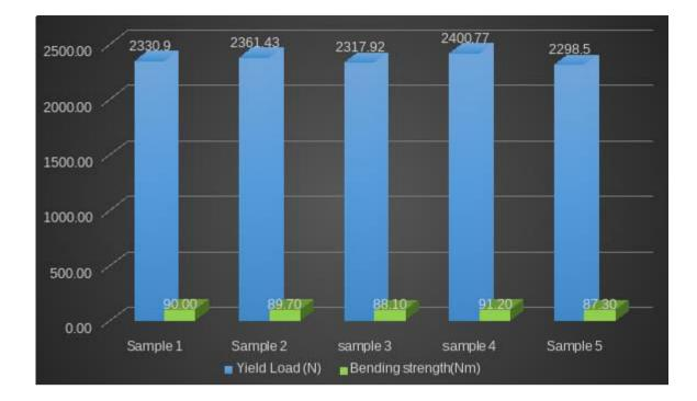
The Expert Femur Nail Manufactured by M/S Auxein Medical Pvt. ltd. tested as per the test method described in ASTM F1264 for four point bend testing in order to determine the Yield load (N) as well as bending strength under the flexural loading.
