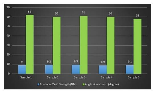
The Metallic Bone screws Manufactured by M/S Auxein Medical Pvt. ltd. tested as per the test method described in ASTM F543-17 for torsional strength.
