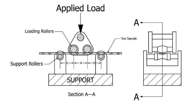
The Metallic Bone plates Manufactured by M/S Auxein Medical Pvt. ltd. tested as per the test method described in ASTM F382-17 for four point bend testing in order to determine the Yield load (N) as well as bending strength under the flexural loading.
