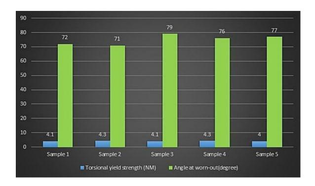
The Metallic Bone screws Manufactured by M/S Auxein Medical Pvt. ltd. tested as per the test method described in ASTM F543-17 for torsional strength.
