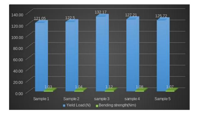
The Metalic Bone plates Manufactured by M/S Auxein Medical Pvt. ltd. tested as per the test method described in ASTMF382 for four point bend testing in order to determine the Yield load (N) as well as bending strength under the .
