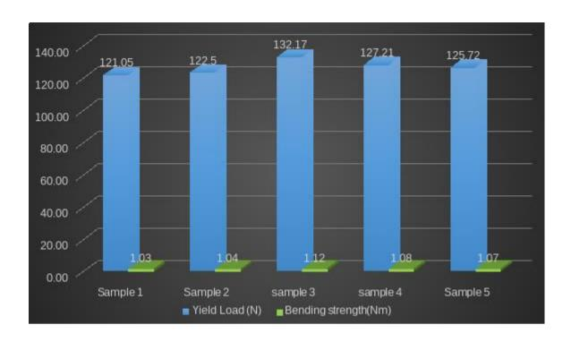
The Metalic Bone plates Manufactured by M/S Auxein Medical Pvt. ltd. tested as per the test method described in ASTMF382 for four point bend testing in order to determine the Yield load (N) as well as bending strength under the .
