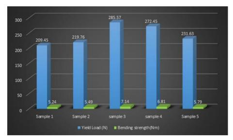
The Metallic Bone plates Manufactured by M/S Auxein Medical Pvt. ltd. tested as per the test method described in ASTM F382-17 for four point bend testing in order to determine the Yield load (N) as well as bending strength under the flexural loading.
