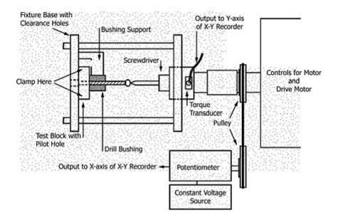
The Metallic Bone screws Manufactured by M/S Auxein Medical Pvt. ltd. tested as per the test method described in ASTM F543-17 for insertion/removal torque.
