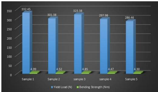
The Metallic Bone plates Manufactured by M/S Auxein Medical Pvt. Itd. tested as per the test method described in ASTM F382-17 for four point bend testing in order to determine the Yield load (N) as well as bending strength under the flexural loading.
