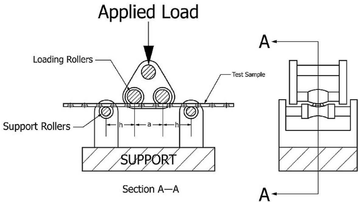
The Metallic Bone plates Manufactured by M/S Auxein Medical Pvt. Ltd. tested as per the test method described in ASTM F382-17 for four point bend testing in order to determine the Yield load (N) as well as bending strength under the flexural loading.
