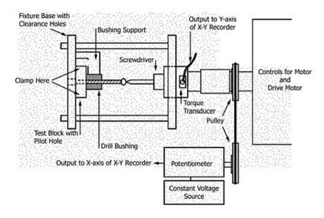
The Metallic Bone screws Manufactured by M/S Auxein Medical Pvt. ltd. tested as per the test method described in ASTM F543-17 for torsional strength.
