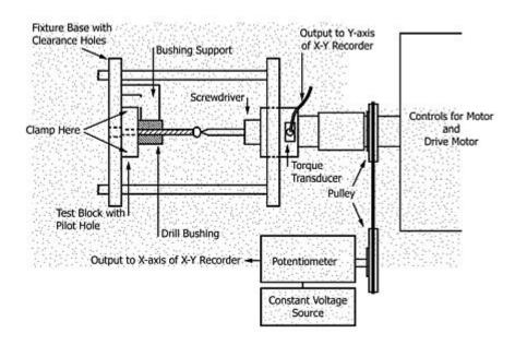
The Metallic Bone screws Manufactured by M/S Auxein Medical Pvt. ltd. tested as per the test method described in ASTM F543-17 for torsional strength, axial pull strength insertion/removal torque.
