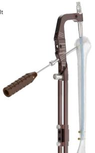
**Jig Removal from the nail:** After the final proximal locking has been achieved, the jig has to be detached from the nail. Use the socket wrench S11 **(10-1199.00)** to remove the connecting screw from the nail and separate the jig from the nail.
