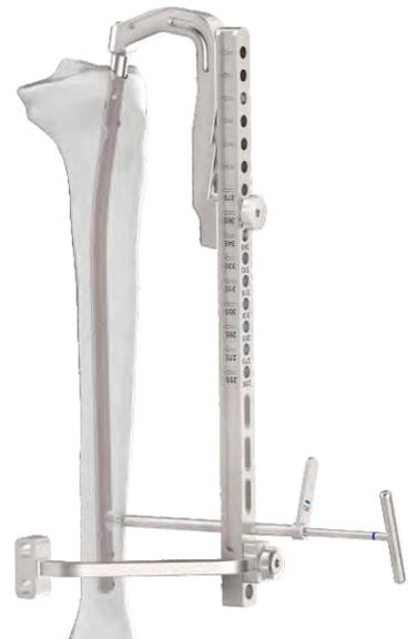
**Nail repositioning:** Pass the Ø5.2mm Drill sleeve (520-028) through the hole in the Distal aiming device for the positioning rod and advance it until it sits flush with the bone. Through the drill sleeve pass the Ø5.2mm Drill with T-Handle (520-030) until it reaches the slot on the nail. Remove drill bit and drill sleeve. Through the positioning rod hole insert the positioning rod (520-031) and secure it in place using the stabilizing device (520-032).
